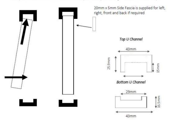
Panels lift and drop into place, with the larger U Channel placed across the top. Side fascias are supplied, and if required these can be glued, taped or pinned in place. Once the side fascias are fitted, the panels cannot lift out without first removing the fascias, so we recommend only installing them if necessary.
